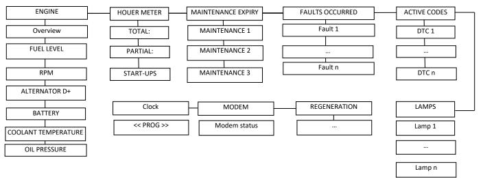
To move between instrument groups, use the RIGHT\_BUTTON and the LEFT\_BUTTON. To move between instruments inside a group, use the UP\_BUTTON and DOWN\_BUTTON. If an instrument is disabled or inactive, it is not displayed. E.g.:
