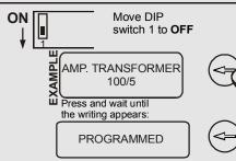
Having programmed the Ammeteric Transformer the PUMP OVERCURRENT threshold is automatically adjusted to 100% of the nominal Ammeteric Transformer value
